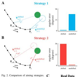
Fig. 2. Comparison of aiming strategies. (A) Strategy 1—aim from the most recently perceived visual feedback, which is four timesteps old. (Left) Hypothetical trial under Strategy 1. When applied to the current cursor position (unshifted), the aim-from-feedback velocity command (solid blue arrow) would result in the cursor (blue circle) missing the target (green circle) by 23°. (Right) Hypothetical results
